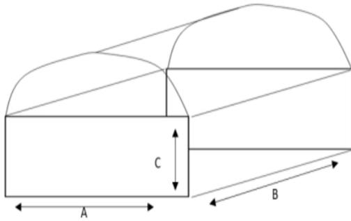
$$\text{Surface Area} = 2(A \times C) + 2(B \times C) + \frac{\pi}{2}(A \times B) + \pi\left(\frac{A^2}{4}\right)$$
