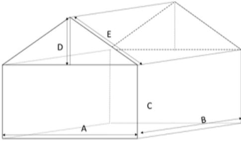
$$\text{Surface area} = 2(A \times C) + 2(B \times C) + 2(E \times B) + AD$$
